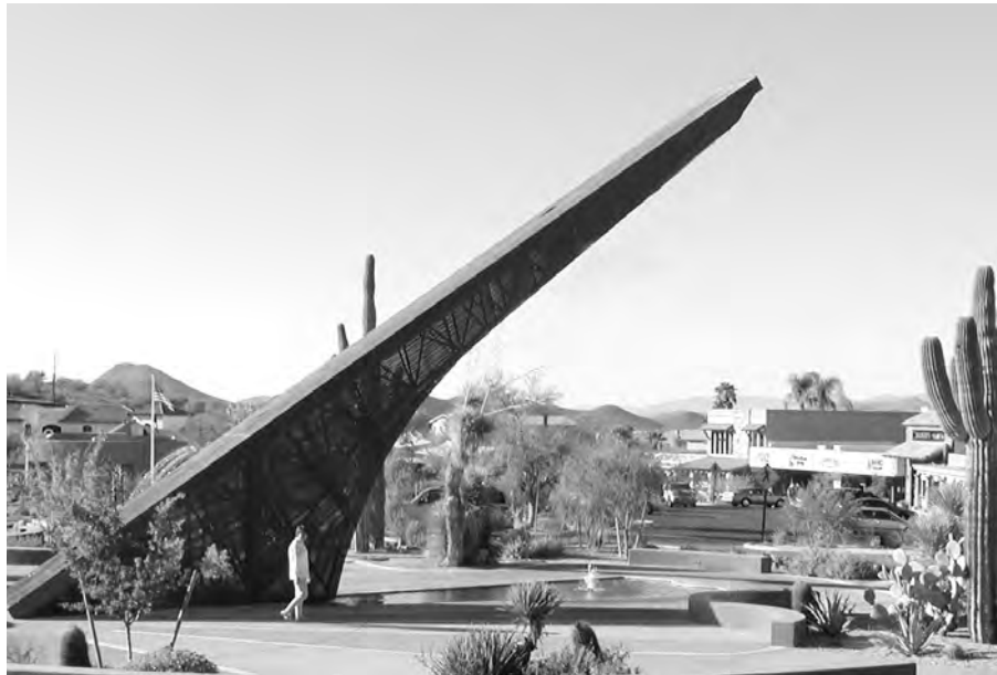
Figure 25-2 Solar time can be measured with a sundial. The long arm of the sundial (the gnomon) casts a shadow on the dial's horizontal face. The movement of the shadow is used to measure the passage of time. Solar noon occurs when the shadow points exactly north. This is the largest sundial in the United States, located near Phoenix, Arizona.
